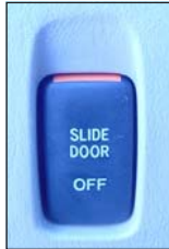
Switch OUT: Power Functions Enabled
